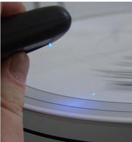
If you use the *Speed Light* (AC039) you can reach an even higher or more accurate adjustment, completely independent of the power line or frequency of your country. As well, the 300 Hz calibrated light, used as an external light source is completely independent from possible power line fluctuations, which could influence the result by regular light. The 300 Hz of the *Speed Light* are generated by a stabilized quartz oscillator and permit a very exact adjustment.
